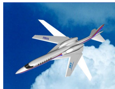
Fig.12 A reference concept of variable geometry SSBJ
